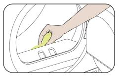
Inside the machine, there are humidity sensors that detect whether the laundry is dry or not.
